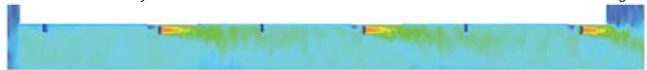
Velocity field induced by the jet fans when only six of the twelve fans are activated.
